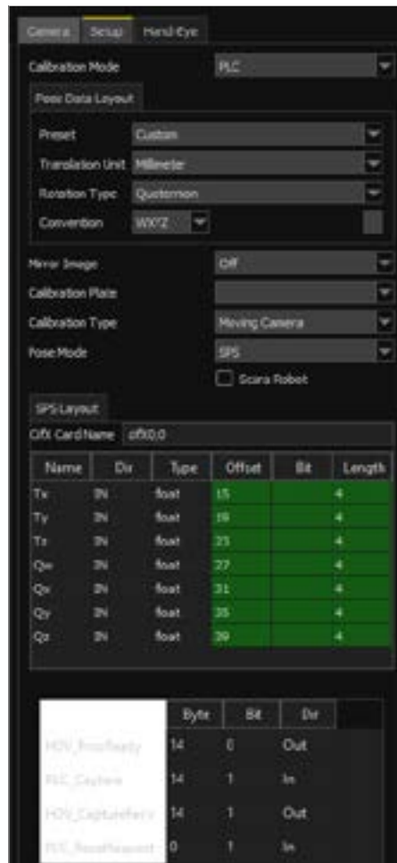
Fig. 43: LumiScan Hand-Eye Calibration: Setup Tab
