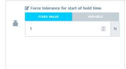
Force tolerance for the transition from search mode to control mode and thus the start of the holding time.
